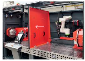
Partition removed by hand for one-station operation
