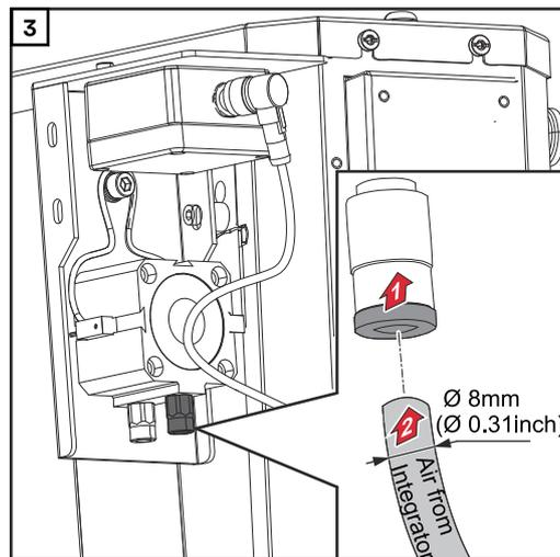
Install compressed air hose from wire cutter
