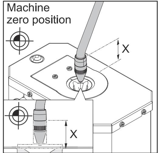
Machine zero position with installed gas nozzle (same as machine zero position with installed Teach-gauge)
