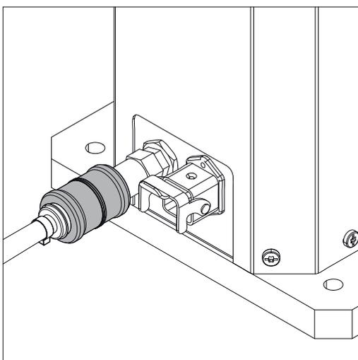
The illustration to the left shows the compressed air relief valve closed = compressed air supply to the device interrupted
