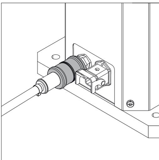
The illustration to the left shows the compressed air relief valve open = device is being supplied with compressed air
